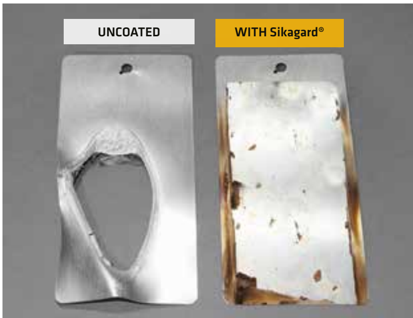
The flame of a Bunsen burner is directed at two identical aluminum plates. The left plate is untreated, the right one is coated with Sikagard®. After 15 seconds, the untreated plate starts to melt in places which would have the potential to start a fire in the vehicle. By contrast, on the right-hand plate treated with Sikagard®, an insulating protective layer is formed. It holds the heat off for at least 30 minutes. In a serious situation, this would give the passengers valuable time to exit the vehicle.
